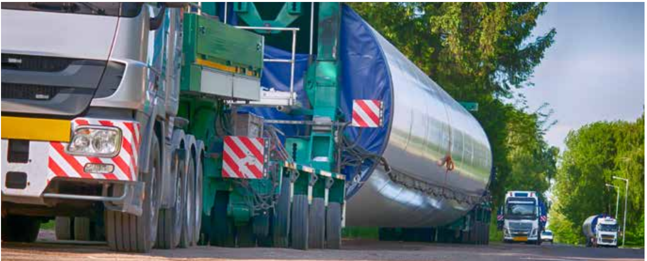
Nb-containing steels for the production of taller, lighter structural supports make possible base diameters that can meet transportation clearance requirements and weight loads that can mitigate transportation and logistics costs, effectively securing a steel solution for taller wind tower demand.
